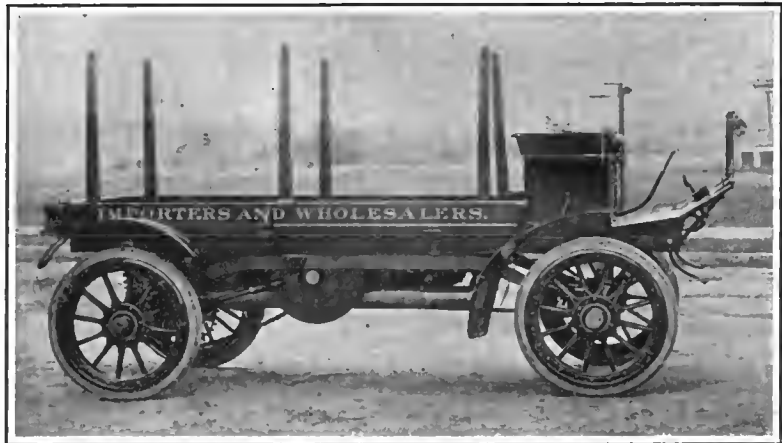
KNOX STAKE TRUCK BODY ON REGULAR DOUBLE-CYLINDER CHASSIS.
